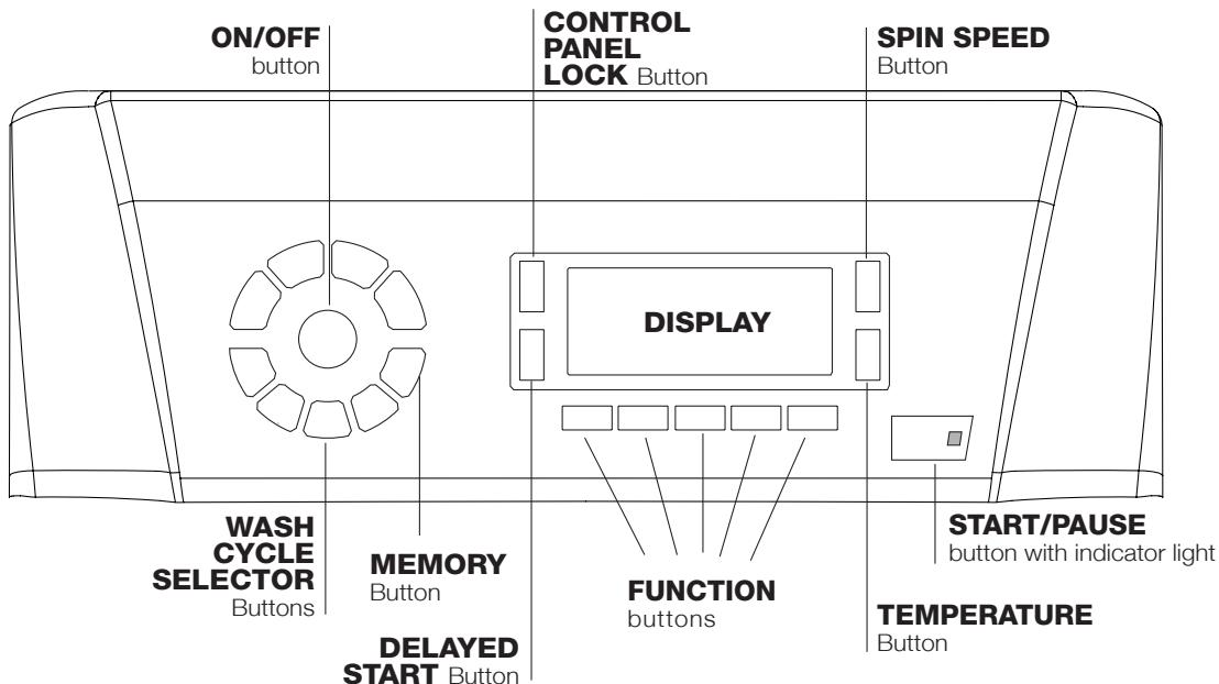
**ON/OFF** button : press this briefly to switch the machine on or off. The START/PAUSE indicator light, which flashes slowly in a green colour shows that the machine is switched on. To switch off the washing machine during the wash cycle, press and hold the button for approximately 2 seconds; if the button is pressed briefly or accidentally the machine will not switch off. If the machine is switched off during a wash cycle, this wash cycle will be cancelled.
